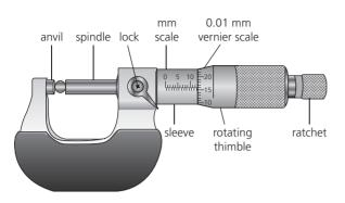
Turning the ratchet moves the spindle until it just touches the object. The ratchet then slips to avoid deforming the object.
