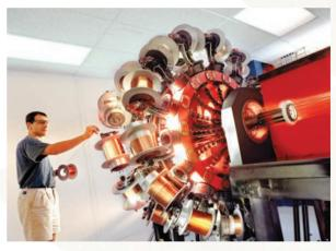
Physicists need to solve problems, such as design problems. This machine weaves superconducting wire into cable to produce powerful superconducting electromagnets for accelerators.
