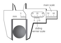
The reading in mm is taken from the position of the zero on the sliding scale. Here this is between 24 and 25. The next significant figure (to 0.1 mm) is found by judging which scale mark on the sliding scale is perfectly aligned with a mark on the main scale. Here this is 5. The reading is 24 + 0.5 = 24.5 mm.
