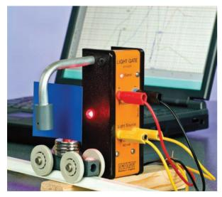
A motion experiment using a light gate
