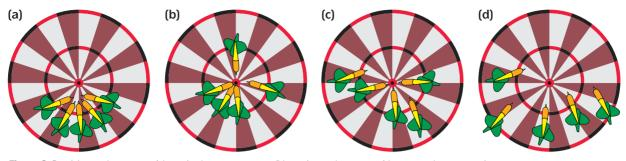
*Figure 8 Precision and accuracy: (a) precise but not accurate; (b) precise and accurate; (c) accurate but not precise; (d) neither accurate nor precise.*
