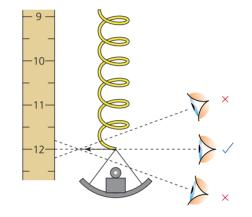
Figure 5 Try to position your eye close to the scale and look in the correct direction to avoid parallax errors.
