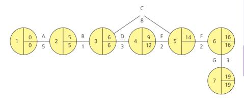
**Figure 2.9.2** CPA for the production of a table lamp base (Table 2.10.2)
