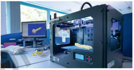
Figure 1.7.8 FDM machines print 3D models from 3D CAD drawings.
