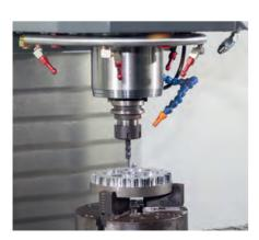
**Figure 1.7.4** Milling machines can drill holes, cut slots or shape a range of materials.
