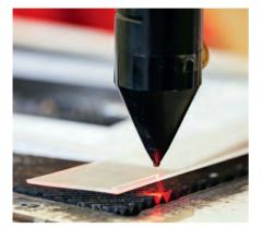
**Figure 1.7.2** CAD drawings can be converted to a CNC program, which controls laser cutters.
