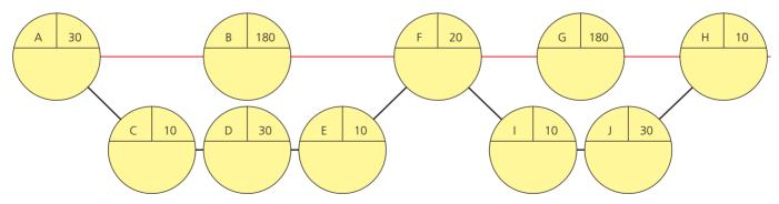
Figure 2.9.1 Critical Path Analysis of making a cup of tea
