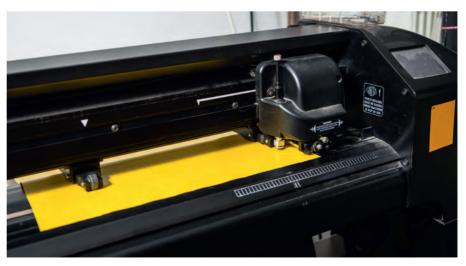
**Figure 1.7.6** Plotter cutters convert 2D CAD drawings into a CNC program to cut out from sheet materials.
