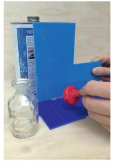
**Figure 1.4.4** Solvent cement is used to join polymers such as acrylic, ABS and PVC.
