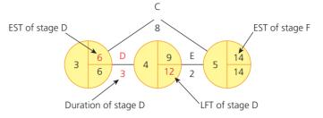
**Figure 2.9.3** Each node shows the earliest start time (EST) and the latest finish time (LFT) for the previous stage
