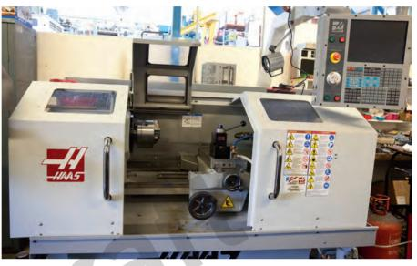
Figure 1.7.5 CNC lathes can be used to reduce metal bars or plastic rods, and for thread-cutting and boring.
