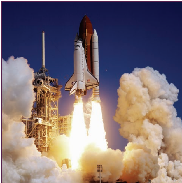
Figure 3.2 The space shuttle accelerating away from its launch pad. The force needed is provided by several rockets. Once each rocket has used all its fuel, it will be jettisoned, to reduce the mass that is being carried up into space.
