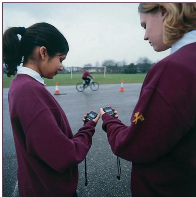
Figure 2.2 Timing a cyclist over a fixed distance. Using a stopwatch involves making judgements as to when the cyclist passes the starting and finishing lines. This can introduce an error into the measurements. An automatic timing system might be better.
