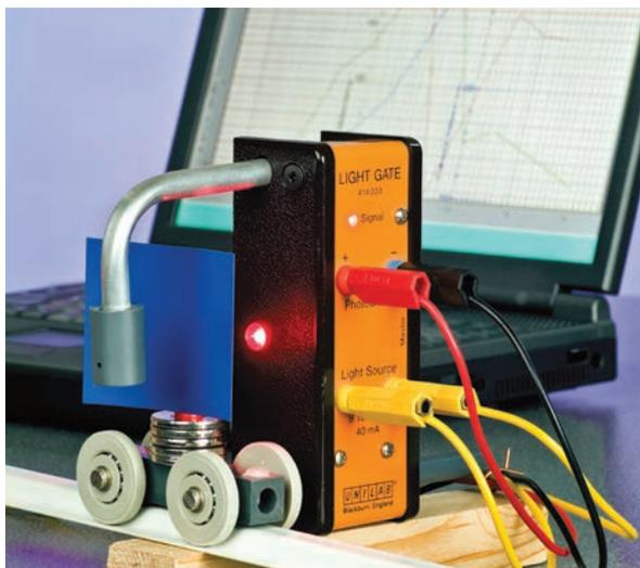
A motion experiment using a light gate
