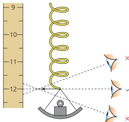
**Figure 5** Try to position your eye close to the scale and look in the correct direction to avoid parallax errors.
