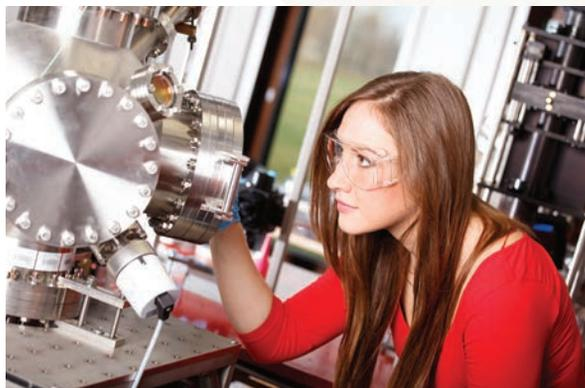
Physicists need to apply their knowledge when using practical equipment. This is a laser deposition chamber, in which a laser beam evaporates material in order to coat another surface.
