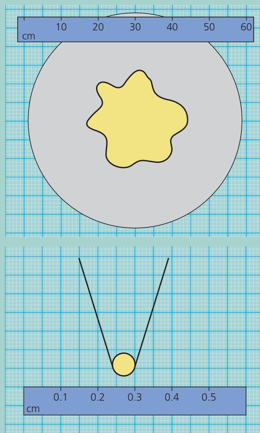
Figure A2 Volume of the drop = volume of the oil film = area of the oil film  $\times$  thickness of the film
