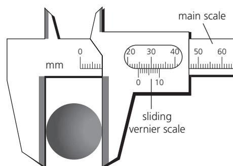
The reading in mm is taken from the position of the zero on the sliding scale. Here this is between 24 and 25. The next significant figure (to 0.1 mm) is found by judging which scale mark on the sliding scale is perfectly aligned with a mark on the main scale. Here this is 5. The reading is  $24 + 0.5 = 24.5 \text{ mm}$ .
