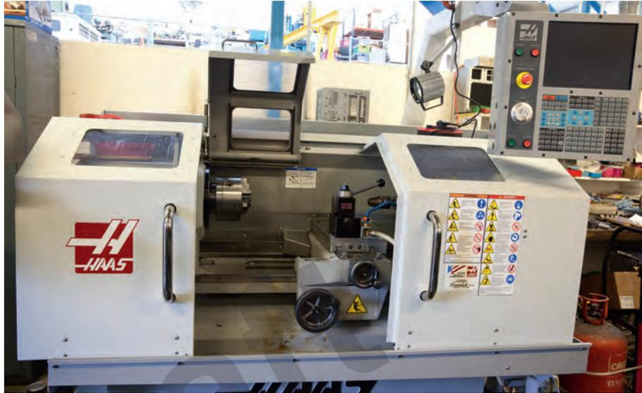
**Figure 1.7.5** CNC lathes can be used to reduce metal bars or plastic rods, and for thread-cutting and boring.
