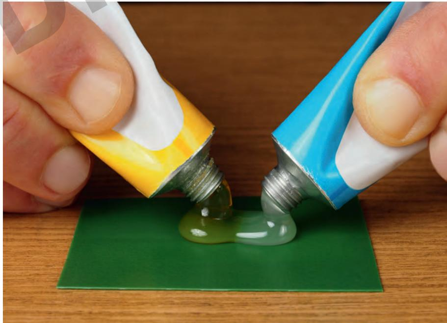
**Figure 1.4.3** Epoxy resin is used to join different materials together.
