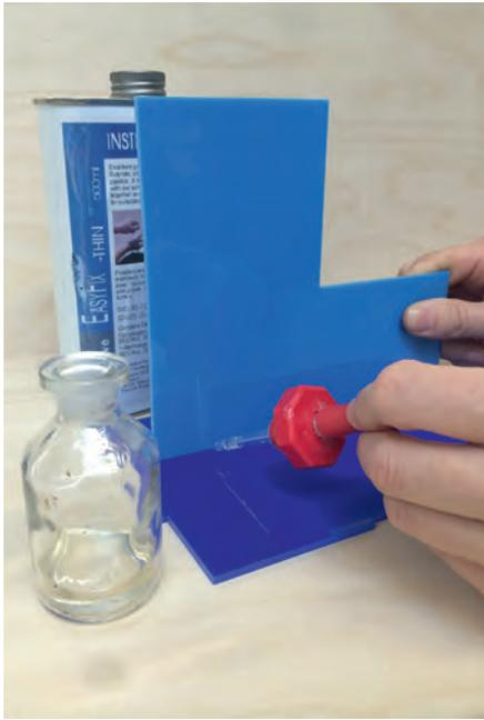
**Figure 1.4.4** Solvent cement is used to join polymers such as acrylic, ABS and PVC.
