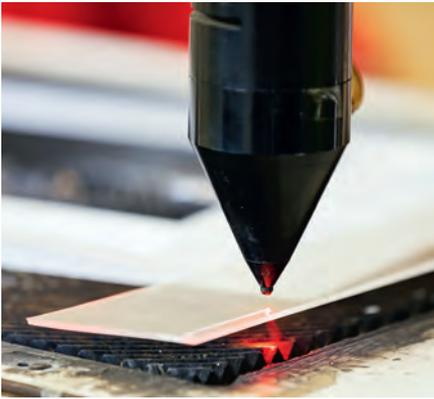
**Figure 1.7.2** CAD drawings can be converted to a CNC program, which controls laser cutters.
